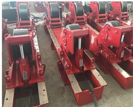
Hydraulic cylinders up / down
