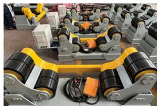
LARGE WIDTH PU WHEELS FOR THIN THICKNESS VESSELS
